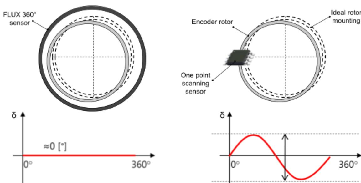
Sensor geometry causes FLUX encoders to inherently average out eccentricity across the circumference of the rotor, resulting in significant reduction in eccentricity error. However, a sensor with a "one-point" scanning capability will exhibit eccentricity errors [δ] over a complete rotation in the form of a sinusoidal wave.
