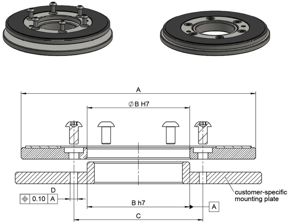
Fig.4.2.: GMI Angle Rotor (GAR) mounting using ID sliding fit
