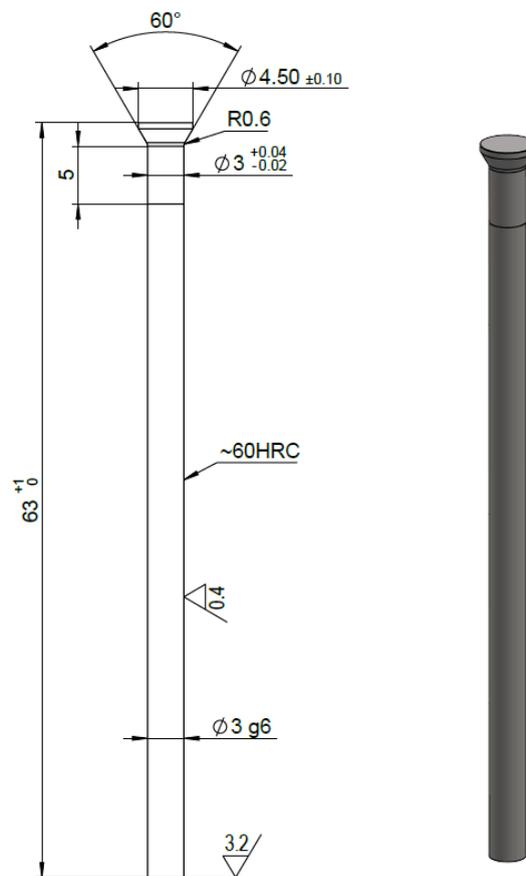
Fig.11.2.: Dowel pin DP-3g6-63 dimensions
