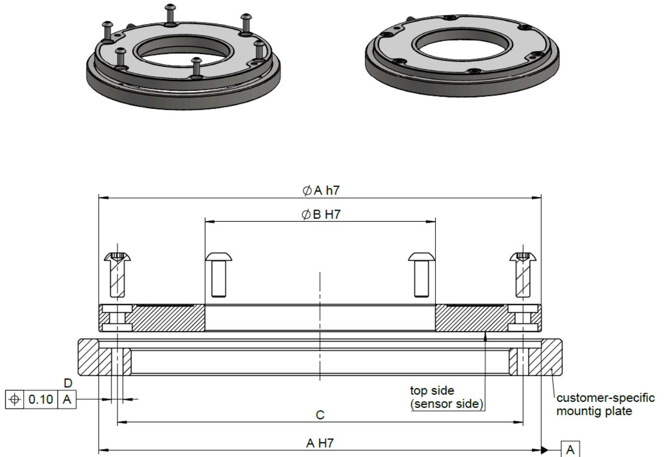
Fig.4.3.: Stator (GAS) mounting using OD sliding fit
