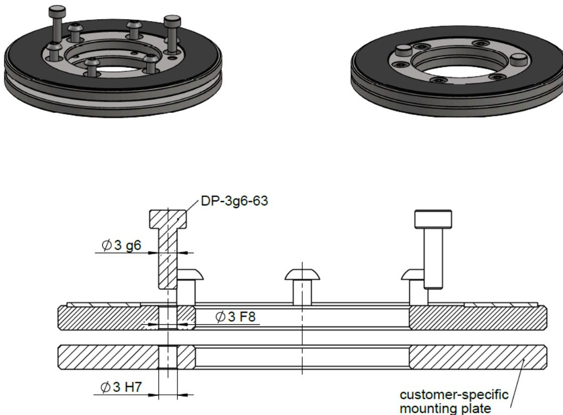
Fig.4.6.: GMI Angle Rotor GAR Dowel-Pin mounting
