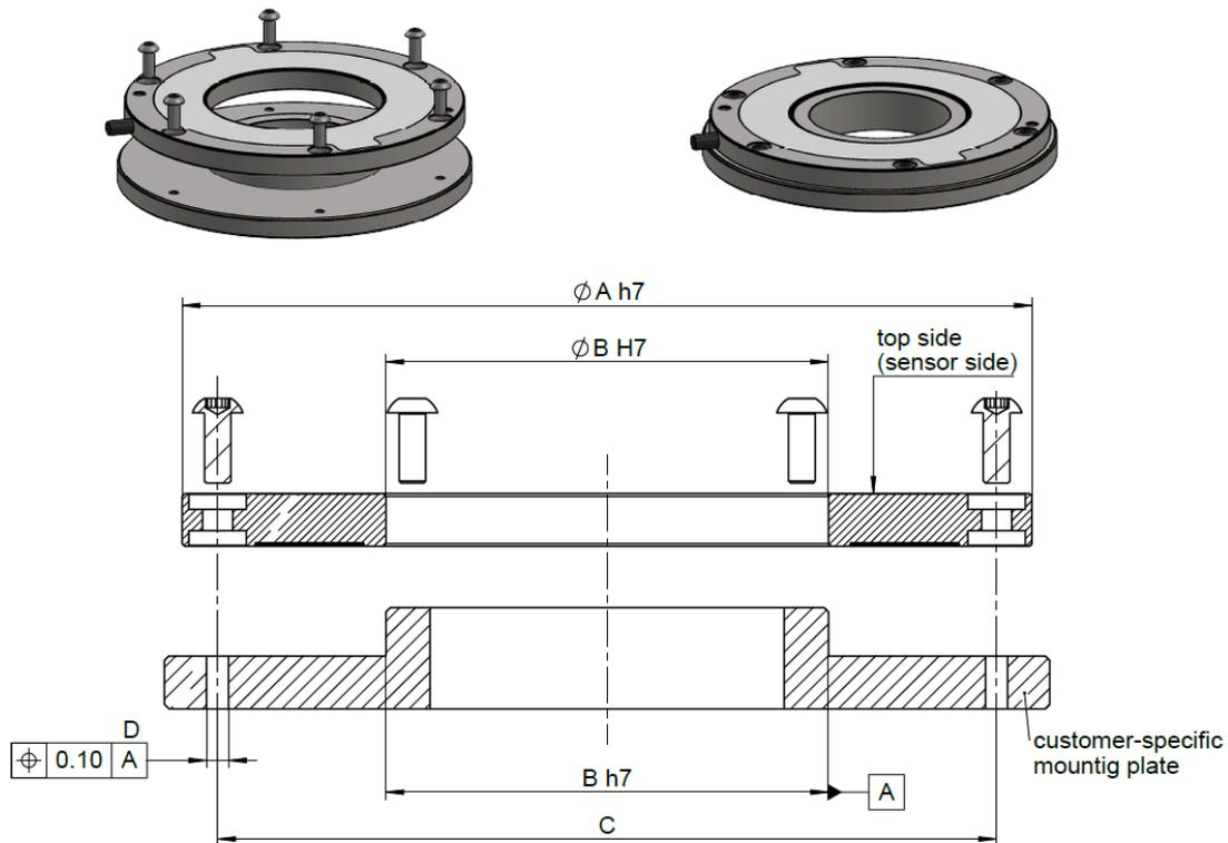
Fig.4.1.: GMI Angle Stator (GAS) mounting using ID sliding fit
