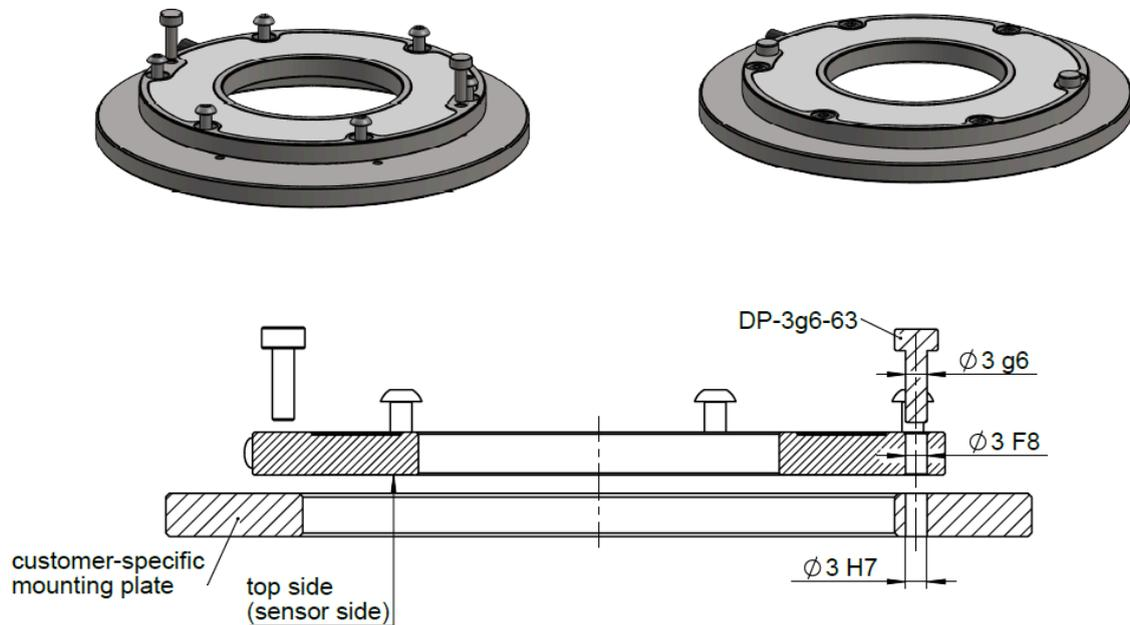
Fig.4.5.: GMI Angle Stator GAS Dowel-Pin mounting
