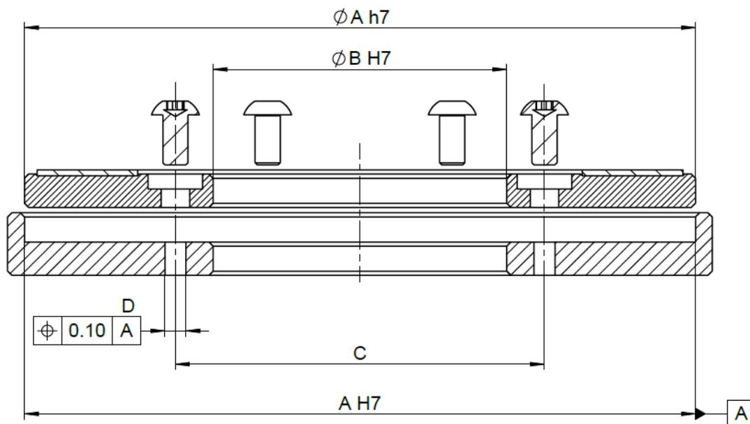
Fig.4.3.: Rotor (GAR) mounting using OD sliding fit
