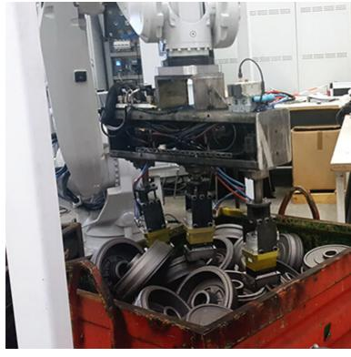
Robot bin picking has is increasingly used in industrial environments. Those heavy work tasks, done by robot, guarantee continuous operation at the strategic beginning of an industrial manufacturing line. When the parts to pick are made of ferromagnetic material, magnet grippers are the key technology.
