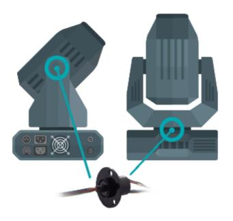
Moving head projectors are more and more used in theatres and shows. These devices must be resistant and extremely flexible and so able to solve all kind of problems faced by lighting engineers on a daily basis. For this reason, these projectors are equipped with a wide range of motors to maneuver them when quiet, smooth and highspeed movements, such as the ones of tilt, pan, and focus, are required.
