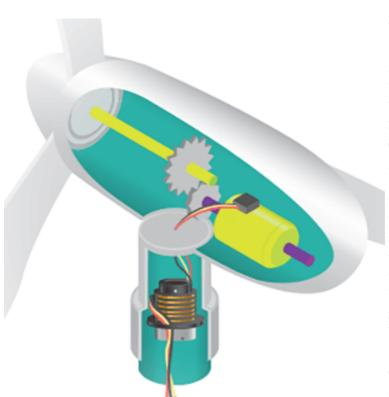
In this particular case, the energy generated by the small size and low voltage wind turbines from the electric generator (aboard the rotating pod) need to be transferred to the land.Slip ring are the best solution in order to avoid any cable twist while passing through the pylon.
