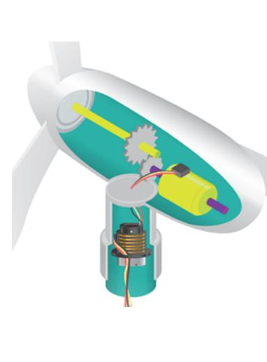
In this particular case, the energy generated by the small size and low voltage wind turbines from the electric generator (aboard the rotating pod) need to be transferred to the land.Slip ring are the best solution in order to avoid any cable twist while passing through the pylon.
