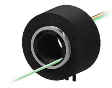
Slip ring for transmission of electrical power and/or electrical signals with through hole for shaft or rotary union. E1M/E1G option comes with an Ethernet channel (100BASE-TX or 1000BASE-T) over a Cat5e cable and 0P1/0P2 option offers an integrated pneumatic rotary joints and 6 to 24power circuits.
