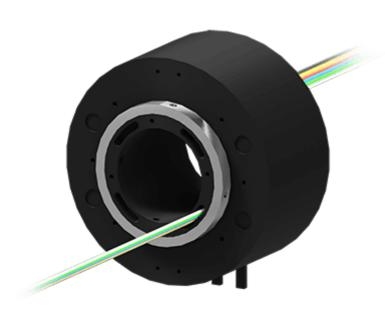
Slip ring for transmission of electrical power and/or electrical signals with through hole for shaft or rotary union. E1M/E1G option comes with an Ethernet channel (100BASE-TX or 1000BASE-T) over a Cat5e cable and 0P1/0P2 option offers an integrated pneumatic rotary joints and 6 to 24 power
