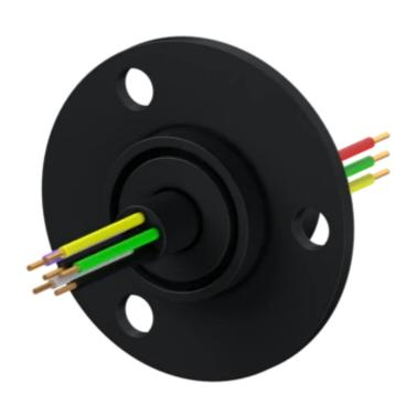
Slip ring specially suited to transmit critical signals, such as hi frequency and data rate, low current and voltages (strain gauges, thermocouples, measuring equipment, etc.) and offering a optionnal fieldbus or Ethernet channel (EtherCAT, Profinet, Profibus, etc.).
