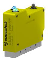
Featuring Variable Field Output (VFO) technology, this automation-ready magnetic gripper can be controlled using CANopen protocols to de-stack and pick single or multiple sheets. Adjustability of magnetic strength between 0 and 100% allows use of this magnet on both thin and thick sheets of varying sizes and material type. CANopen communication allows integration of multiple tools on the same CANopen bus, controlled simultaneously.
