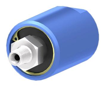
The single passage **SPSM Series** rotary unions are small, lightweight but rugged and corrosionresistant thanks to their aluminum construction with a stainless steel shaft. \* The use of liquid media is not recommended for this product. Please select from one of our other product lines or consult PES if your application requires use of liquid media.
