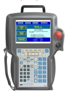
The WeldSaver graphical user interface provides information on device status in real time, with clear visual indicators and descriptions. The interface can be accessed over a network using most JavaScript<sup>TM</sup>-enabled web browsers by entering the working IP address of the device.
