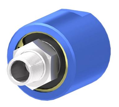
The single passage **SPSM Series** rotary unions are small, lightweight but rugged and corrosionresistant thanks to their aluminum construction with a stainless steel shaft. \* The use of liquid media is not recommended for this product. Please select from one of our other product lines or consult PES if your application requires use of liquid media.
