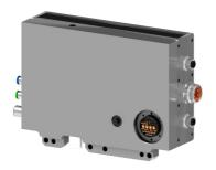
Ethernet/IP control module (3 Control valves, 3 pressure sensors, TC control by remote I/O module, safety sensor "Tool presence", Ethernet/IP connection to tool), 7/8" male 5pins (24VDC), D-Coded M12-4 pins connector (Ethernet/IP) - Rotary Switches: 500 (PGM Mode - IP: 172.29.100.54) - Tool Changer Valves with Output 24VDC.
