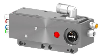
Control module (3 Control valves, 3 pressure sensors, TC control by I/O, safety sensor "Tool presence", Profinet connection to tool), M23-19pins 90° connector, M12-4 pins D-Coded connector (Profinet). Gold plated contacts. Net weight : 1.65 kg. Country of origin : Belgium. HS Code : 84799070.
