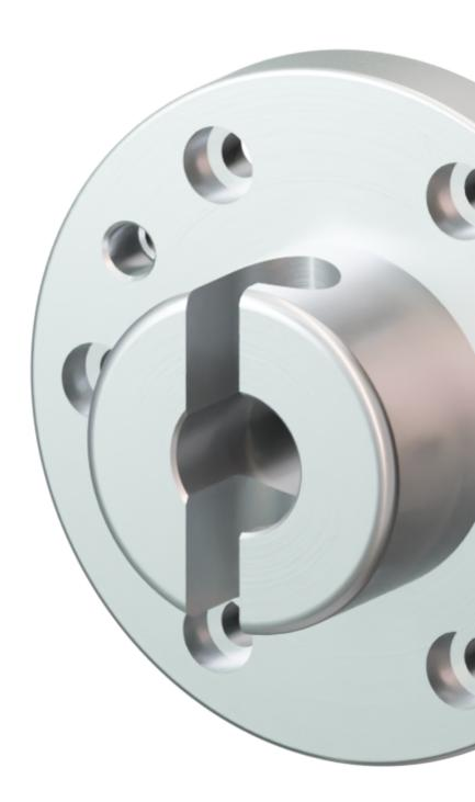
The SWS Connector is our power pack for applications with increased force and torque loads. The semi-cylindrical bolt accurately joins the upper and lower assembly without play. A centering disc can be installed on both the upper assembly (robot side) and lower assembly (tool side) of the robot and ensures that the tools are correctly aligned with the robot arm.
