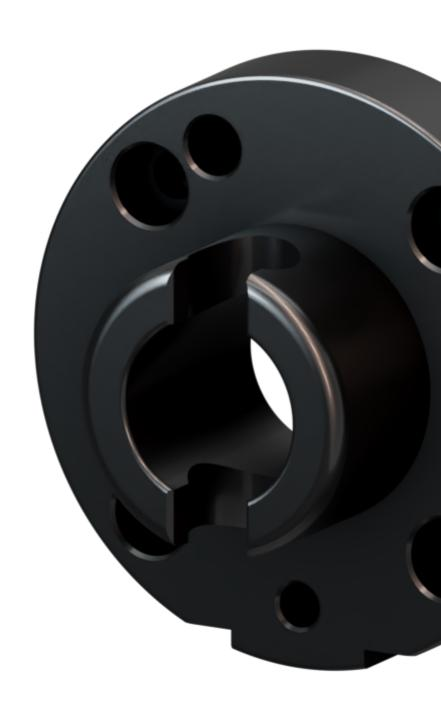
The SHW Connector is a manual tool changer with an optimized locking mechanism. The connector consists of a cylindrical bolt which locks the upper and lower assembly together. A centering disc can be installed on both the upper assembly (robot side) and lower assembly (tool side) of the robot and ensures that the tools are correctly aligned with the robot arm.
